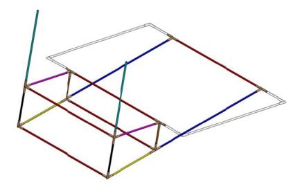
**4.** Add the FL fittings with pipes C and H to complete the frame.
