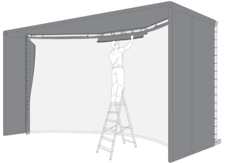
Continue attaching flaps in this manner until you reach the ends. Make any adjustments to center the flaps, still focusing on aligning the bottom edges.
