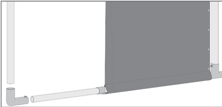
Hold the panel in place with three loose zip ties through the top corner grommets.
