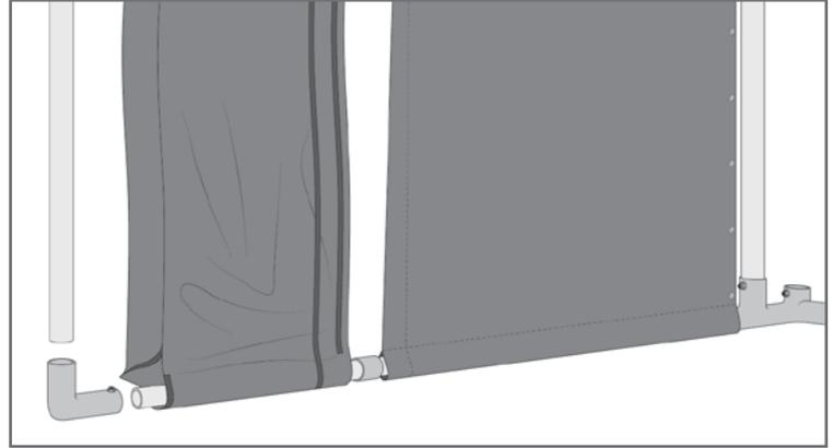
Then, work the front sleeved edge of the wall panel upward onto the front vertical pipe.
