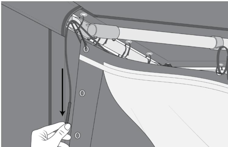
Reattach the turnbuckle, then loosely connect the top and bottom cable ends together on each side via the turnbuckles.
