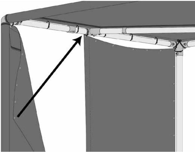
Pull the front and rear wall panels towards each other in the center and connect using the hook-and-loop strips starting at the top. Note you're installing to the closest hook and loop strip, leaving the further strip exposed where the screen will attach.
