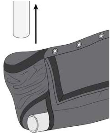
Once both left wall panels are installed, re-install the "L" fitting. Tighten the connector, then attach the hook-and-loop fasteners that wrap around corner.
