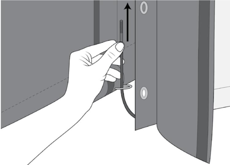
**!** Truth time. Did you orient the collar fittings the way we strongly specified earlier? If there is no U-shaped tab of the collar fitting to feed the cable through, back to the 'Assemble Frame' step you go.
