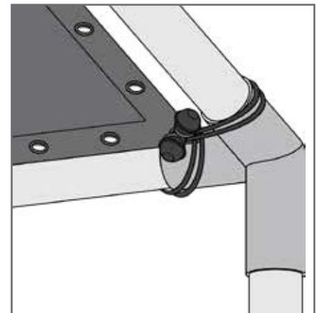
**Only at the four corners** use ball bungees to attach the ceiling to the frame. Use two bungees in each corner grommet (one in each direction).
