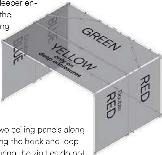
Connect the two ceiling panels along the middle using the hook and loop fasteners, ensuring the zip ties do not interfere with the connection.
