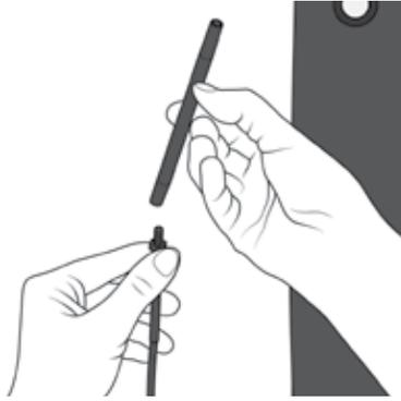
Feed the bottom screen cable upward through collar fitting that you pre-threaded onto the bottom pipe. (You will need to lift the front of the enclosure up to do this.)
