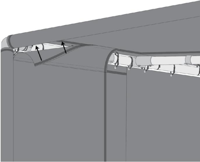
Next, get the wall panel flaps (two identical pieces of narrow black fabric with a pinched sewn pocket at the front).
