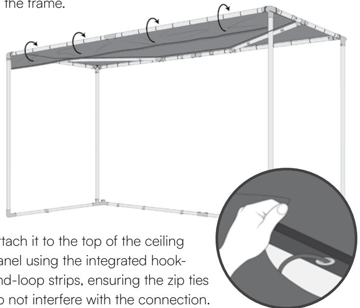
Attach it to the top of the ceiling panel using the integrated hook-and-loop strips, ensuring the zip ties do not interfere with the connection.
