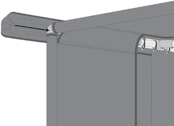
Smoothly attach the flap along the ceiling edge using the hook and loop strips.
