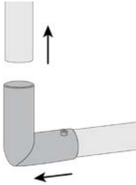
Slide the bottom sleeve of the blue-tabbed panel onto the bottom pipe.
