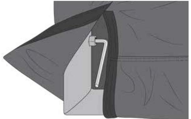
Lift the front panel upward and attach loose zip ties from wall to frame at corners at the top of wall to hold in place.
