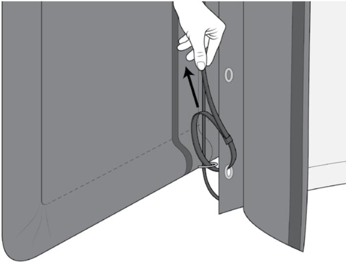
Smooth out the bottom of the screen by pulling the cable tautly thru the bottom collar tabs.
