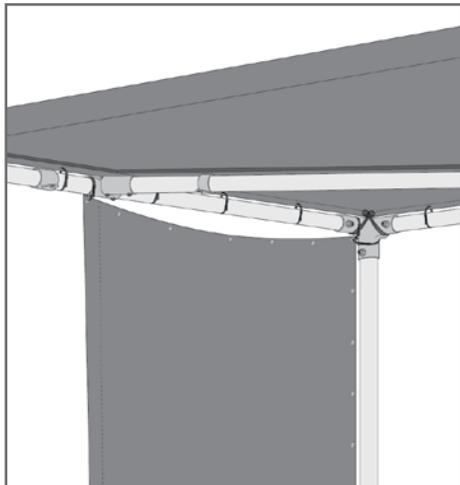
Two zip ties through the rear corner grommet (one around the top pipe, one around the rear pipe). Plus one zip tie around the top pipe at the front.
