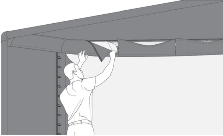
When you get to the end, trim off excess foam using a cutting tool. Make adjustments to smooth out the flaps and tuck in the corners for a neat fit.
